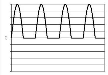
In this case, the average (again, this corresponds to the DC component) is clearly positive, not zero. In fact, if you integrate the signal over one complete cycle, you arrive at
