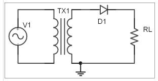
The transformer steps down the voltage, then the diode allows current only when the incoming signal is positive with respect to ground. That current produces a voltage across the load resistor that's one diode drop below the input peak voltage.
